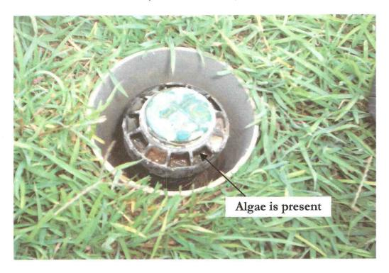
CONDITION OF SPRINKLERS AFTER 10 DAYS OF INSTALLATION (WITH GMX)
