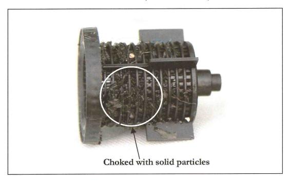
CONDITION OF STRAINER INSIDE THE SPRINKLER AFTER 10 DAYS OF INSTALLATION (WITH GMX)
